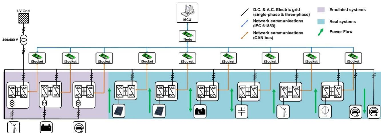
Figure 1. Microgrid connectivity and components.
