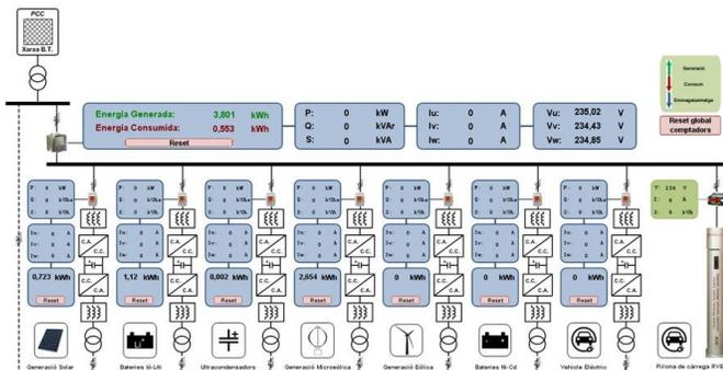
Figure 4. Scada program used for monitoring the microgrid
