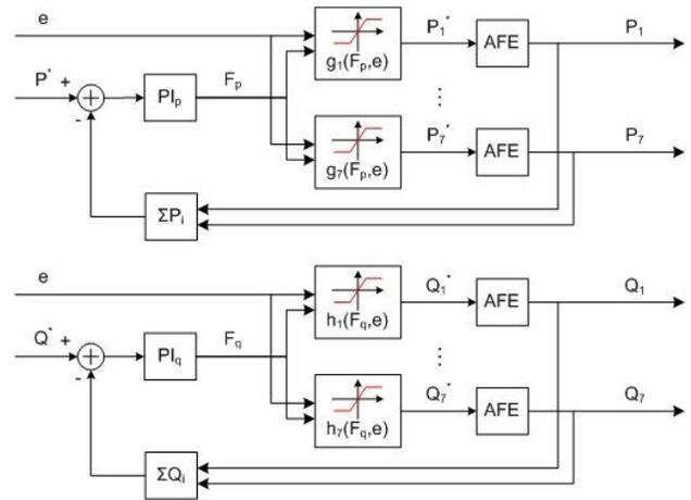
Figure 3. Active and Reactive power closed-loop control.
